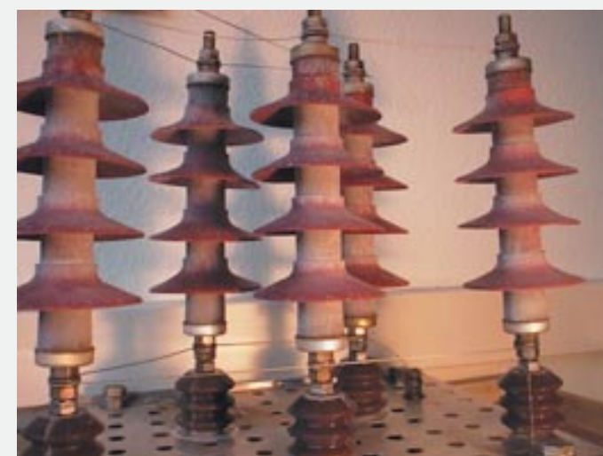
Fig. 1: DEHNmid arrester with considerable salt deposits after a 5000 hours test with cyclically alternating stress including rain, saline fog, temperature fluctuations and UV radiation at a continuous voltage U_c .
