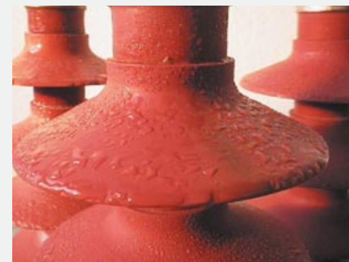
Fig. 2: Regeneration of the water resistance of the arrester already some hours after the stressful 5000 hours test.
