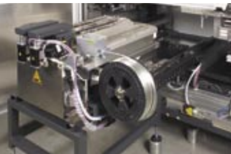
Double wave module in service position
