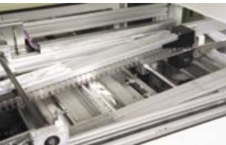
Auto angle adjustment of in-line conveyor
